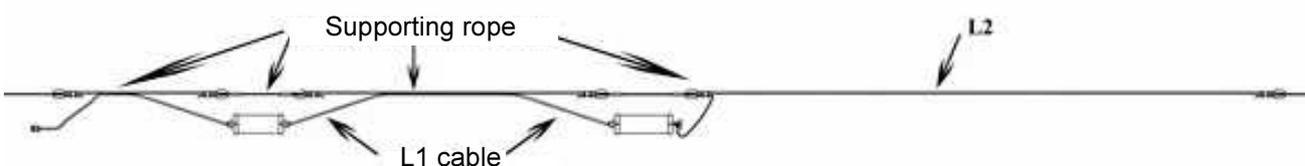
While the excitation of the antenna is made at the same point A the energy is supplied not perpendicularly over the feeder but along the curtain. And the very same cable acts itself as a radiator. There is a choke at the antenna's ending point in order to cut off the current and to provide the antenna with a resonant wavelength. The transformer is used to convert the antenna radiation resistance of 250-300 $\Omega$  to the standard cable impedance of 50 $\Omega$ .
